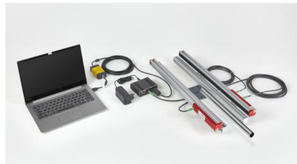
Fig 3: SLM Components of portable system
